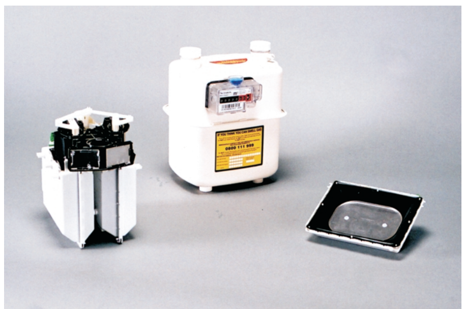
► Meter Engine, U6 meter, and Diaphragm in pan
